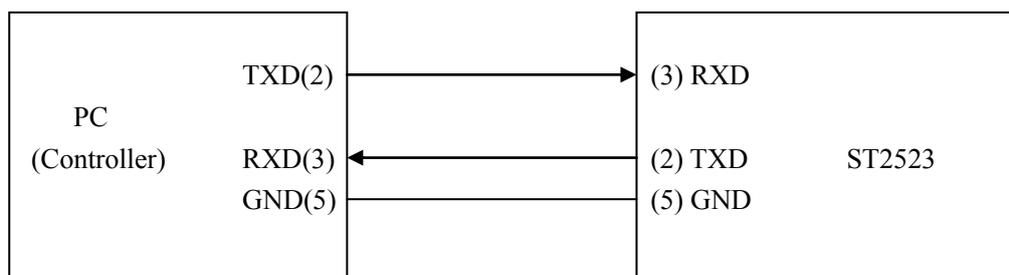
Figure 6-1 Connection of the instrument with a PC
